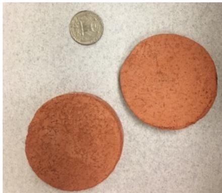
**Figure 3.1.** Ceramic filter disks used for laboratory testing
