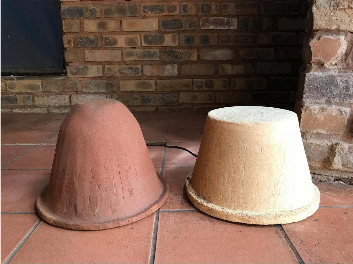
**Figure 4.1.** Filters produced at the production facilities. Left is from the Mukondeni Pottery Cooperative and the right is from the Dertig Production Facility.
