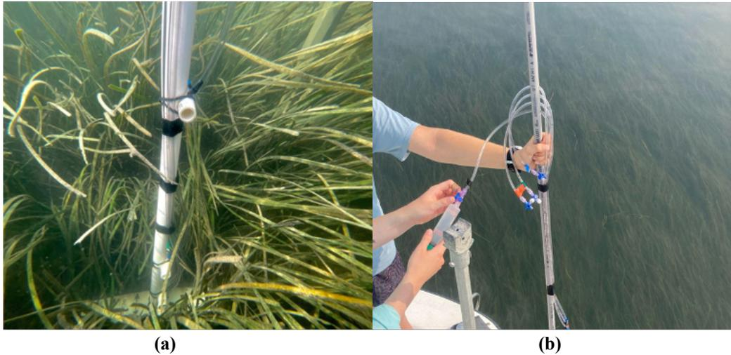
**Figure 2.** a) Shows the sampler used to collect water column samples at 1, 5, 15, and 45 cm from the bottom through the depicted ports. b) Shows the top of the sampler and the syringe used to pull samples up the plastic tubing in 60mL increments.
