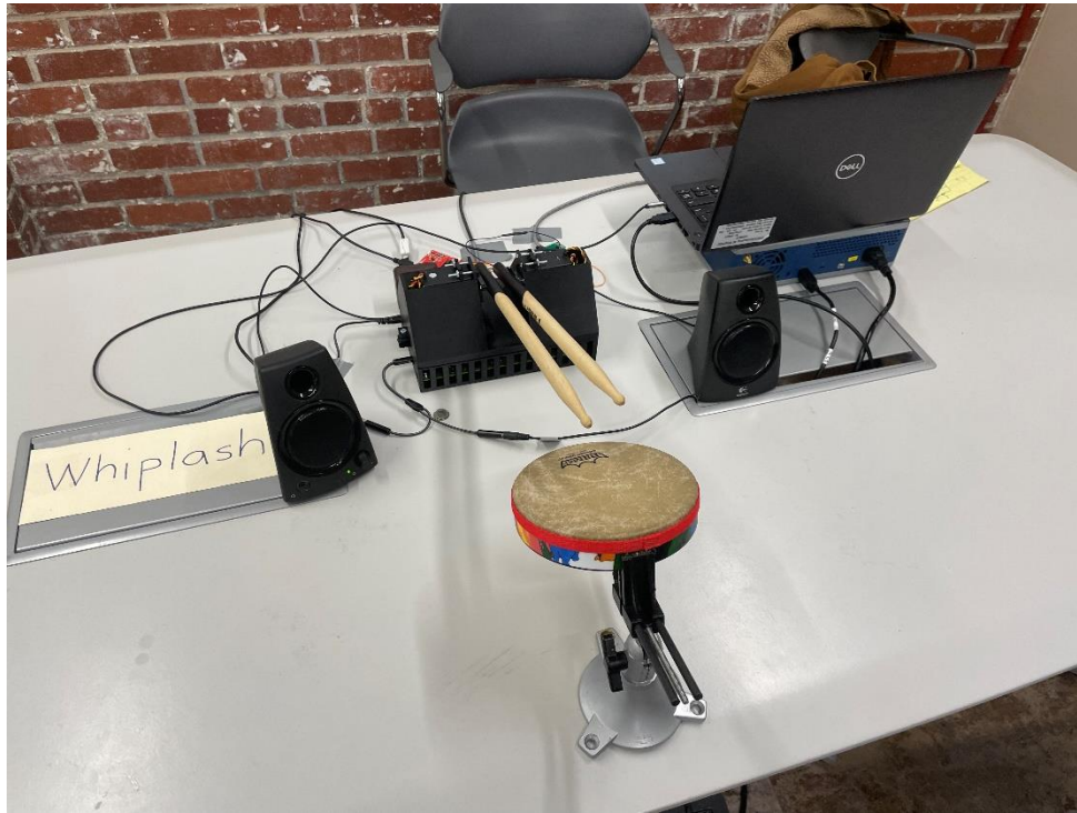
Figure 2: Whiplash Drum Device, this device is able to take in a piece of musical audio, parse out the beat, and play a physical drum to the beat of the song (Anselmo, 2022)
