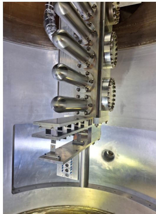
(b) A front-on view of the target ladder with the solid targets in view in the bottom portion of the image.
