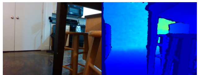
Fig. 3: Images provided by the RealSense D435 camera showing both an RGB image (left) and the depth view of the same scene generated by its depth cameras (right).
