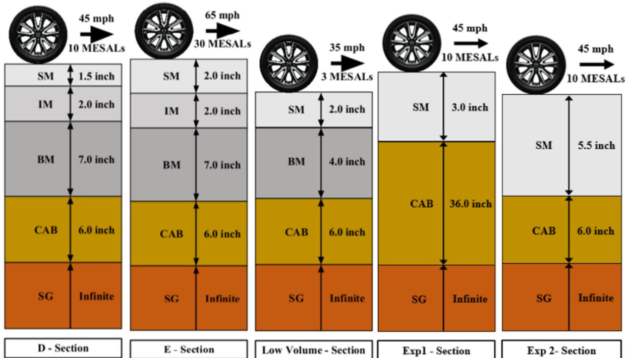
**Figure 5. Asphalt Roadway Cross-sections Used in Analysis**
