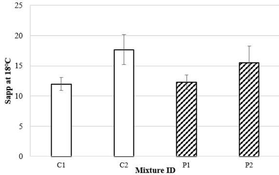
**Direct Tension Cyclic Fatigue Test: S<sub>app</sub>.**
