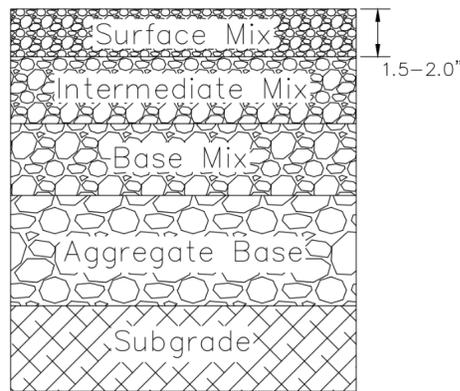
**Figure 3. Typical Asphalt Pavement Cross Section**
