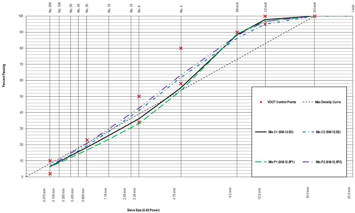
**Figure 7. Aggregate Gradation of Asphalt Mixture Samples.**
