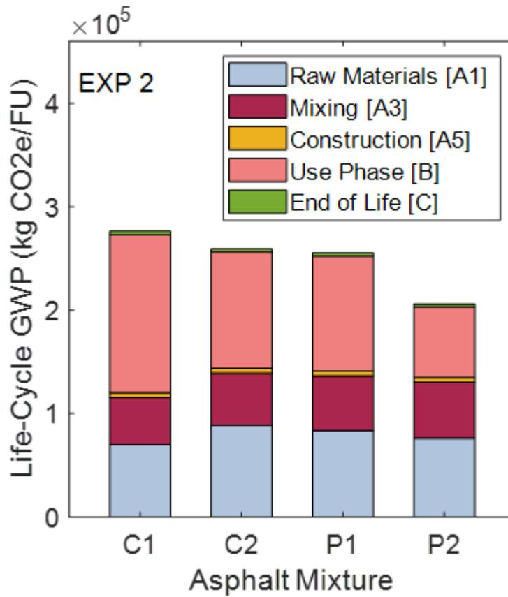
**Figure 23. LCA GWP impacts per Phase for Exp2-Section.**
