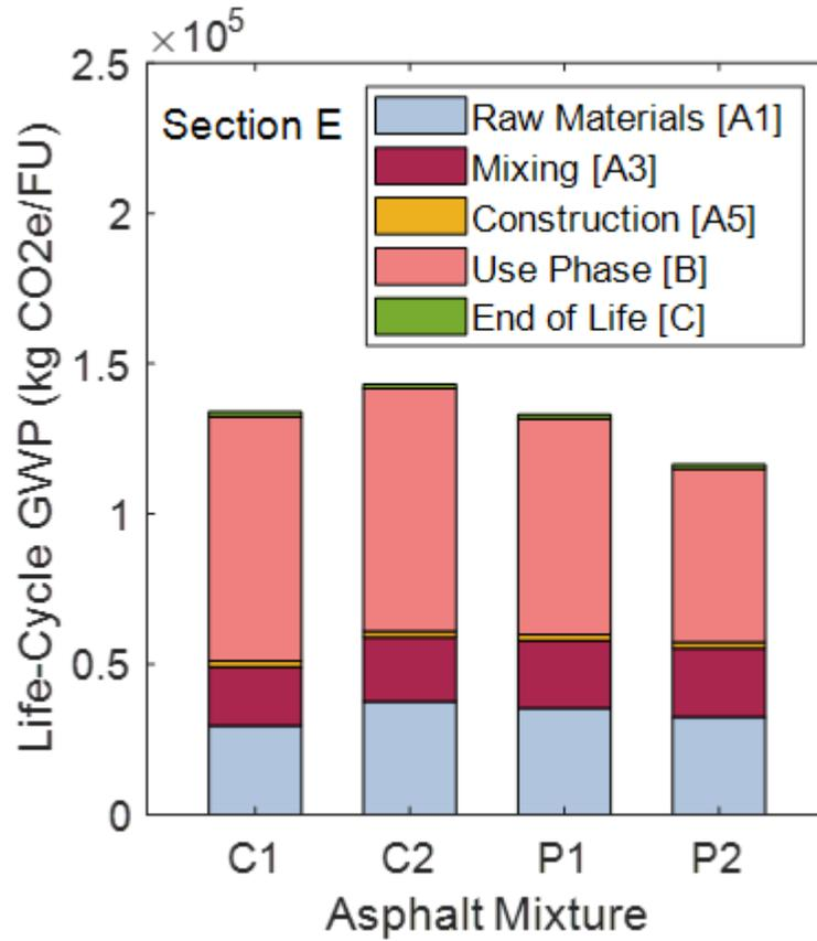
**Figure 20. LCA GWP Impacts per Phase for E-Section.**
