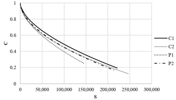
**Direct Tension Cyclic Fatigue Test: C vs. S Curve.**
