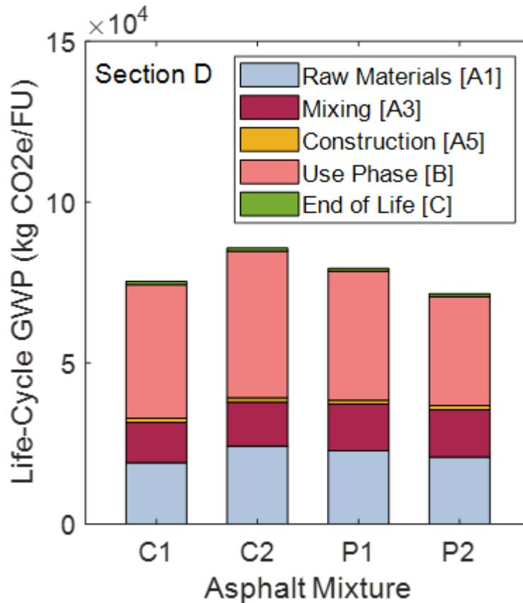
**Figure 19. LCA GWP Impacts per Phase for D-Section. Note that GWP magnitudes are graphed  $\times 10^4$ , unlike all other figures, in which GWP is graphed to  $\times 10^5$ .**
