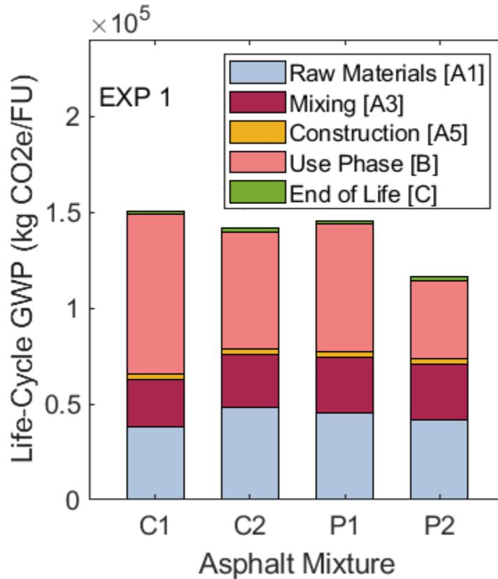
**Figure 22. LCA GWP Impacts per Phase for Exp1-Section.**
