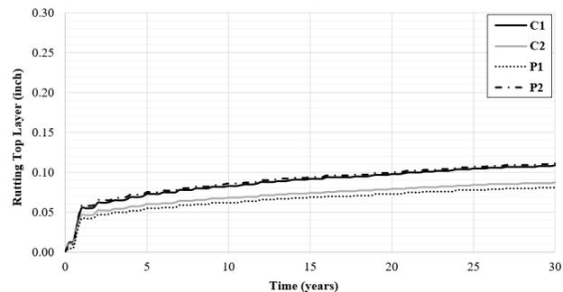
**Figure 18. Rutting Curve for D-Section.**
