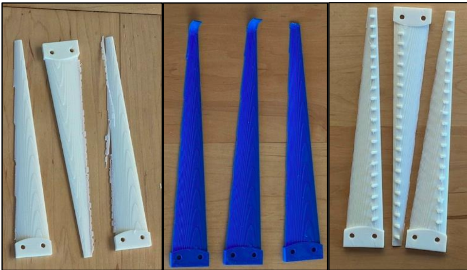
Figure 4. The initial set of modified blade prints to illustrate low quality; pictured from left to right: serrations, folded tips, nodes.
