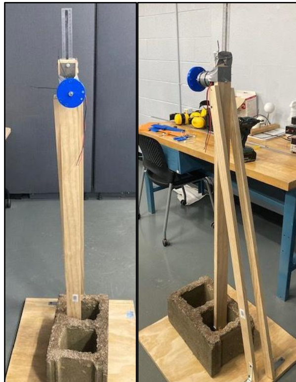
Figure 6: Testing stand with attached hub.
