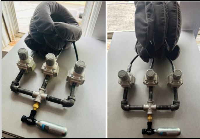
Fig. 1. Final Prototype Assembly. The two images display the airbags inflated to various pressures, connected to pressure regulators, piping system, manual inflator valve and gas cartridge.
