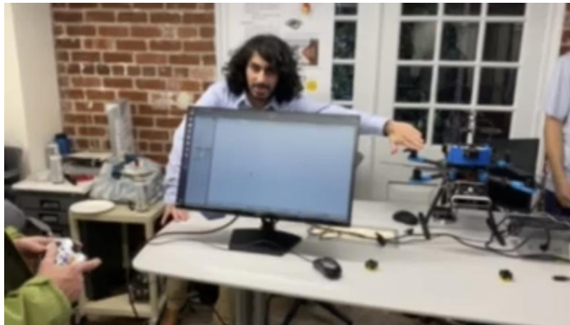
Figure 23. Blocking the right sensor causes the drone to move to the left regardless of input
