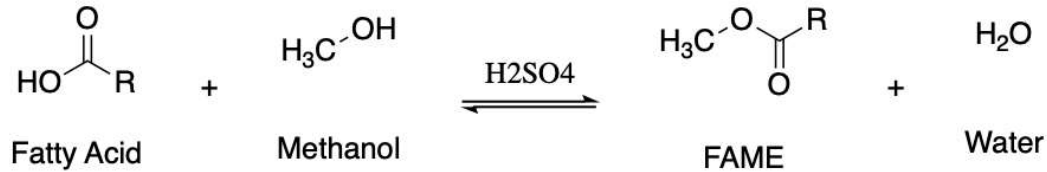
Figure 3.7-01: Esterification of free fatty acids into FAME.
