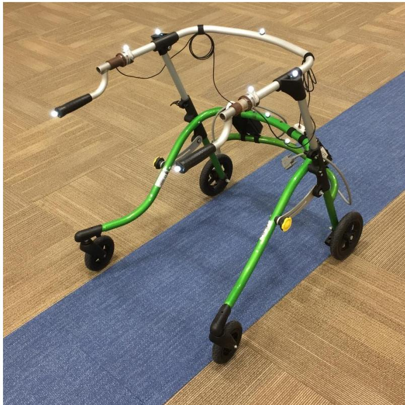
**Figure A.2:** Modified Nurmi Neo Posterior Pediatric Walker used for all manual walker trials with attached load cells for collection of handle reaction force data.
