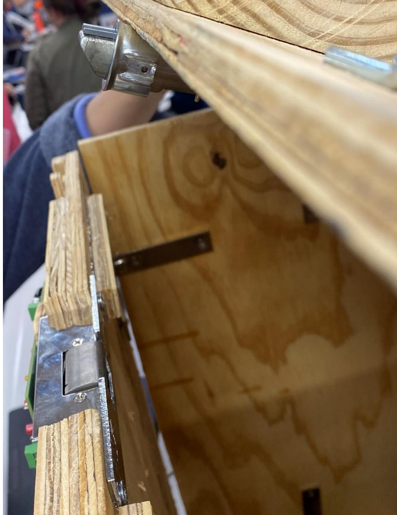
Figure 53 Side-View of Package Box Locking Mechanism
