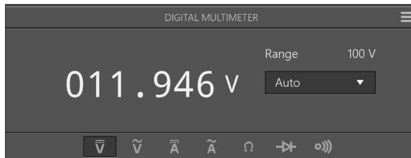
Figure 31 Voltage out of 12V Linear Regulator
