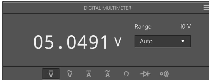
Figure 32 Voltage out of 5V Switching Regulator
