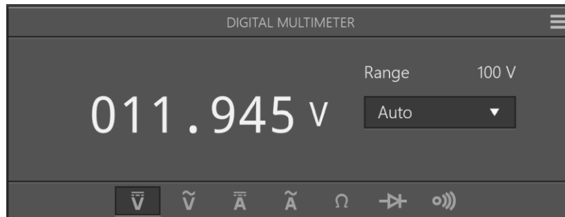
Figure 33 Voltage into Positive Terminal of Electric Strike
