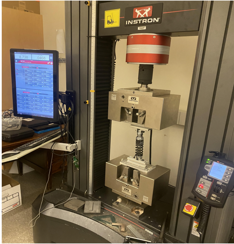
Figure 14: The Instron pneumatic materials testing device was used for compression testing to verify spring rate and maximum deflection. The spring and maximum deflection were measured to be in accordance with manufacturers specifications at k = 400 \text{ lb/in} and \delta = 2.4 \text{ in}
