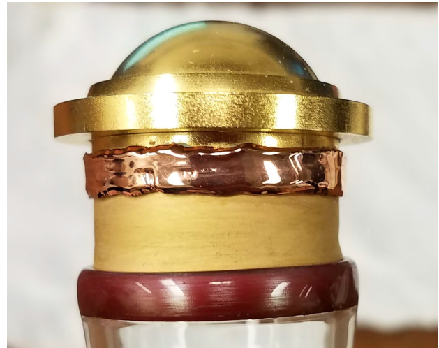
(b) The copper covering the joint between the plated copper and plated aluminum on the MK-II design (Loretta).
