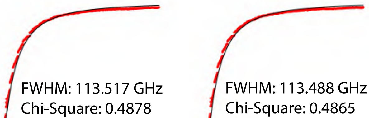
Figure 5.14: A comparison of the Lorentzian fit (left) and a full Lorentzian fit accounting for all possible hyperfine transitions for a RbD2 line measured at 155°C
