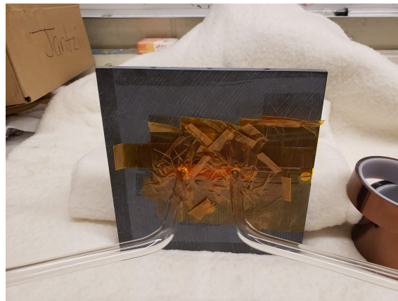
(b) Underside of the oven base, the hole sealed with Kapton tape and aluminosilicate insulation
