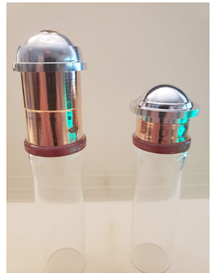
(c) Prototype MK-I (left) and MK-II (right) windows set loosely atop their copper tubes with a glass-to-metal seal. These units have been electropolished, hence their shine.
