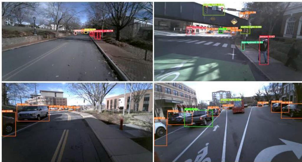
Figure 5: Examples of traffic scene images with predicted bounding boxes.
