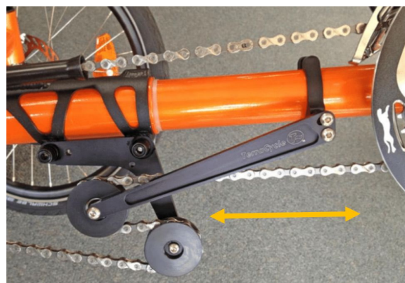
Fig. 1.8: Chain gobbler on a tadpole trike. Each idler wheel is fixed to their respective parts of the telescoping arm. As the arm changes in length, so does the distance between the idler wheels. As a result, the chain remains taut for any length of the arm (Catrike Boom Adjust Chain Tensioner, 2018).
