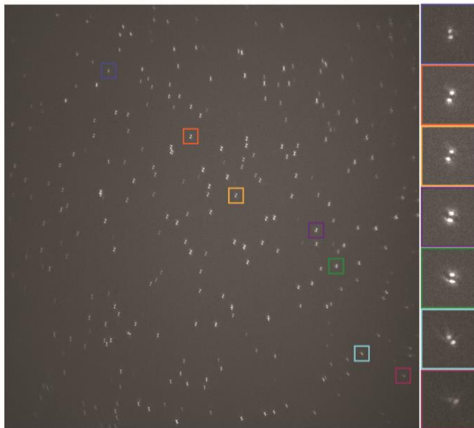
Figure 4.1. DH-PSFs of fluorescent beads depend on position relative to the central imaging axis. On the right are the magnified DH-PSFs in different colored boxes. The fluorescent beads are placed between a coverslip and agarose pad (1.5%, w/v) in PBS. The angle between the two lobes changes as the location of bead changes. For instance, the angle between two lobes of the DH-PSF in yellow box is close to 90^\circ , while the angle of DH-PSF in red box is close to 0^\circ . Note that the angle of DH-PSF in navy blue box is close to 90^\circ , which may be because it is stuck in the agarose pad. Additionally, the intensity of the two lobes and the side lobe pattern change from bead to bead throughout the field-of-view.
