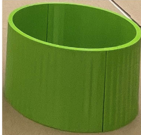
Figure 55. Extended nosecone mold (Height 10 cm)
