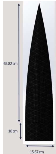
Figure 3. Final ogive nosecone design and dimensions.
