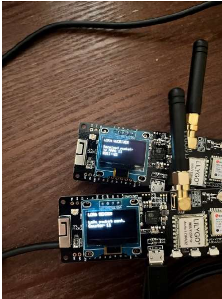
Figure 67. LCD of LoRa receiver module displaying static message (sender module's name) and dynamic message (number of packets sent by sender module)
