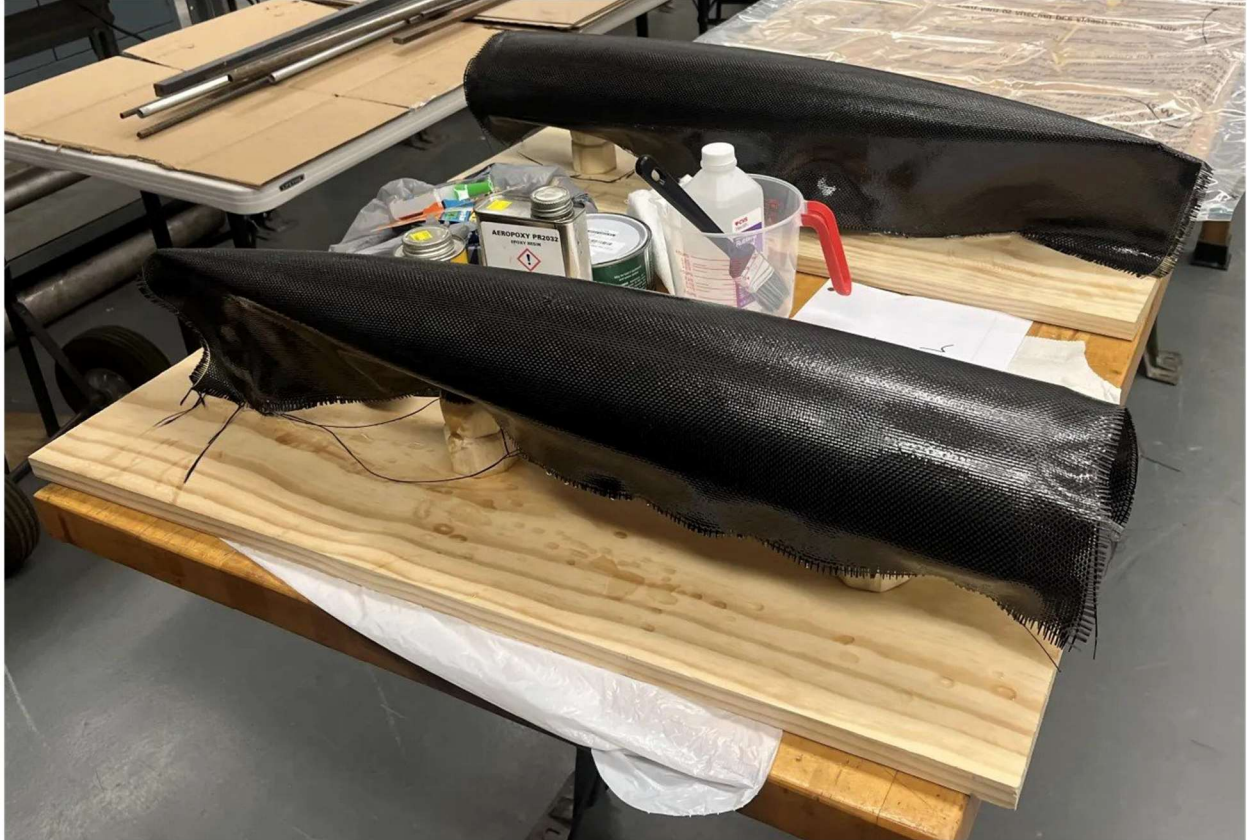
Figure 56. Manufacturing of nosecone using carbon fiber wet layup method
