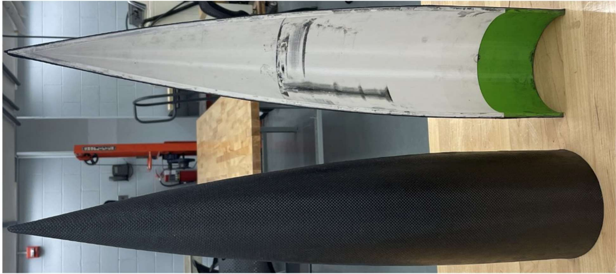
Figure 57. After 3 layers of CFRP wet layup
