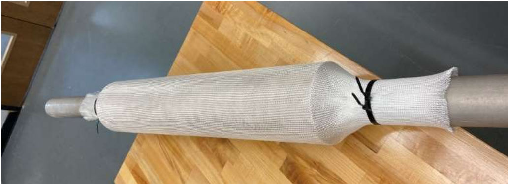
Figure 63. Fiberglass sleeve fixed over phenolic tubing.
