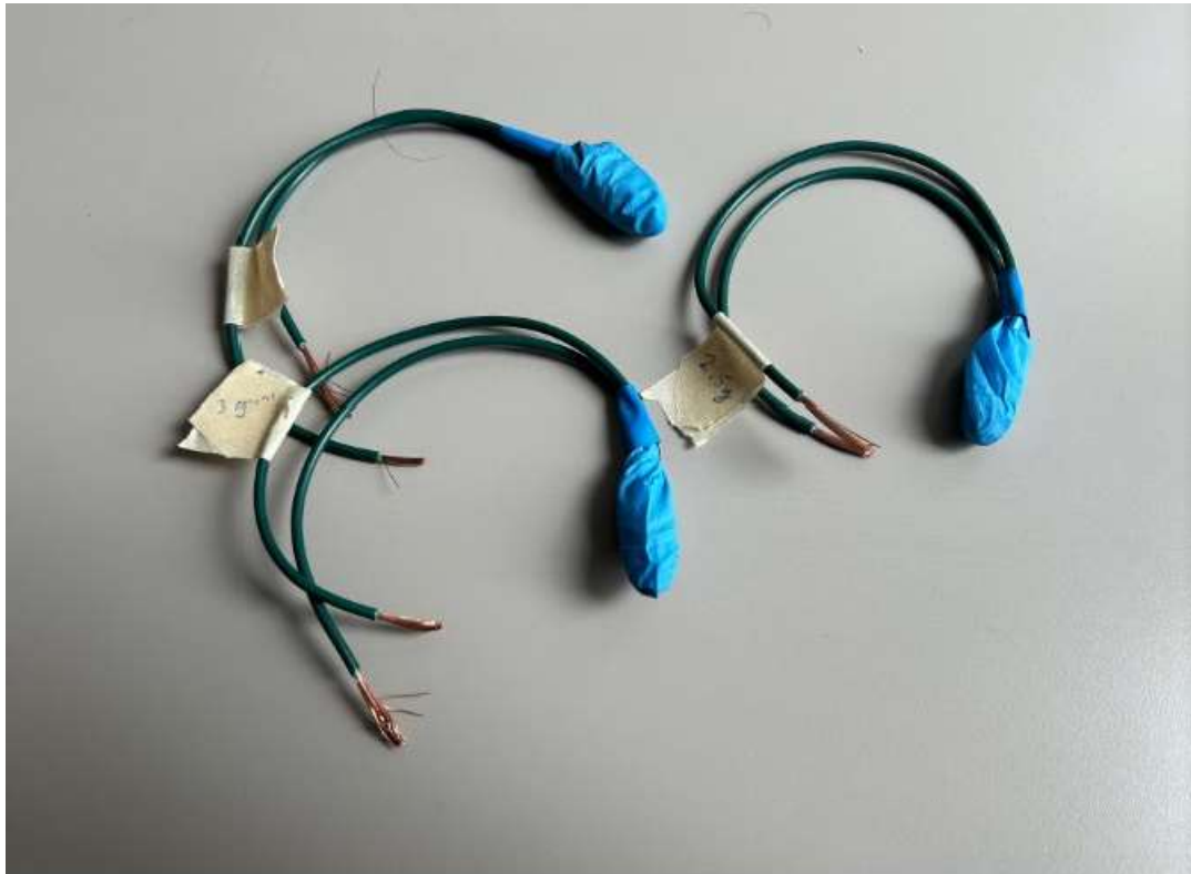
Figure 72. Charges used in final test with spare coupler
