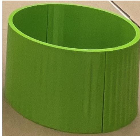
Figure 55. Extended nosecone mold (Height 10 cm)
