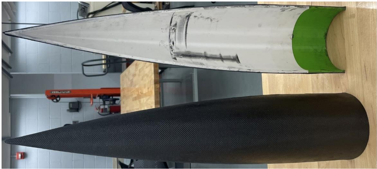
Figure 57. After 3 layers of CFRP wet layup
