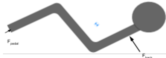
Figure 17: Free body diagram of a rider with reaction forces during pedaling
