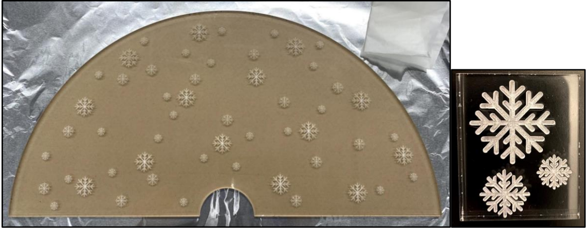
Figure 19: Final acrylic snow sheet implemented into the final assembly, along with the smaller test strip of acrylic used to test etching intensity and snowflake size.
