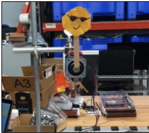
Figure 12: Bipolar stepper motor with microstepper driver with a prototype sun arm attached
