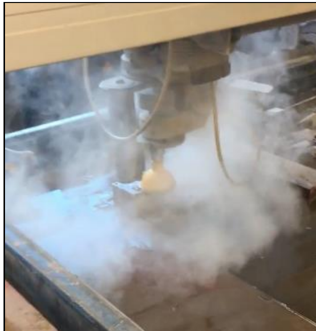
Figure 5. Waterjet Blasting into an Aluminum Block.
