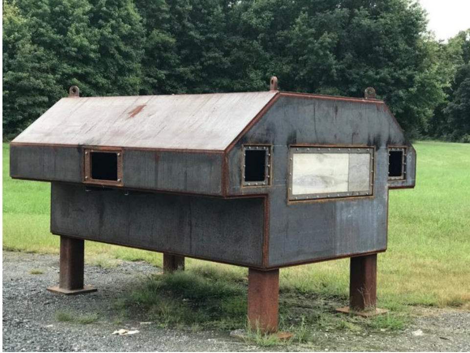
Figure 1.1: Ground vehicle testbed where flame measurements were taken, located at Aberdeen Proving Grounds, MD. Photo courtesy of the U.S. Army Research Lab.
