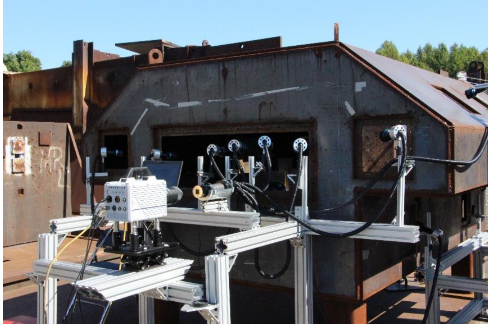
Figure 4.3: Experimental setup of the 4D sensors to visualize flames within the ground vehicle testbed located at ARL APG
