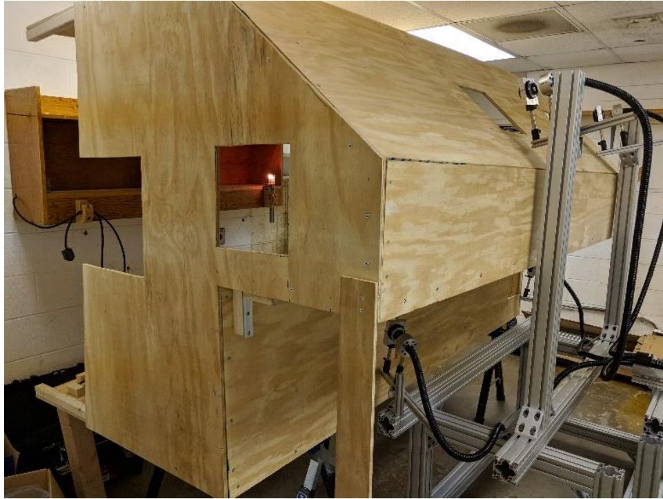
Figure 4.2: Wooden replica of the ground vehicle testbed built at a 1:1 scale used for design and rehearsal of the FBE sensor setup
