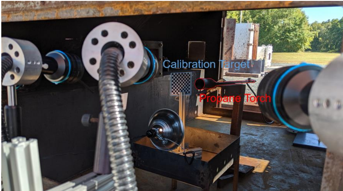
Figure 4.6: The calibration target within the ground vehicle testbed as seen from the outside, also showing the pool container, the propane torch, and some FBE input ends
