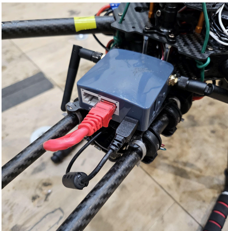
Figure 21. Onboard modem for Raspberry Pi
