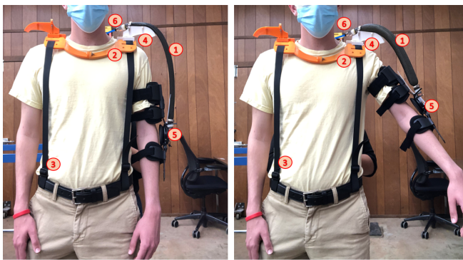
Fig. 13. System Assembly While Idle (left) and Actuated (right) (1) McKibben Style Artificial Muscle (2) A 3D printed shoulder support brace that provides an attachment point for the artificial muscles (3) A strap system that keeps the shoulder brace from sliding out of place and can be adjusted based on the user (4) A 3D printed muscle mount that guides the artificial muscle's expansion direction (5) A purchased arm brace that provides an attachment point on the arm for the bottom end of the artificial muscle (6) Input Air supply to the artificial muscle
