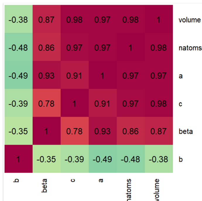
Figure 5.3: Pearson correlation coefficient plot for the dataset comprising 32 \text{RE}_2\text{SiO}_5 compounds. Dark red indicate strong positive correlation. The plot shows that the variables “b” and “volume” are the only two variables that are not highly correlated and thus are not redundant and suitable inputs for the ML model.
