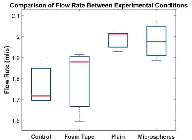
**Figure 3: Flow Rate Analysis.** Each prototype underwent flow rate testing to determine any impact on functionality.
