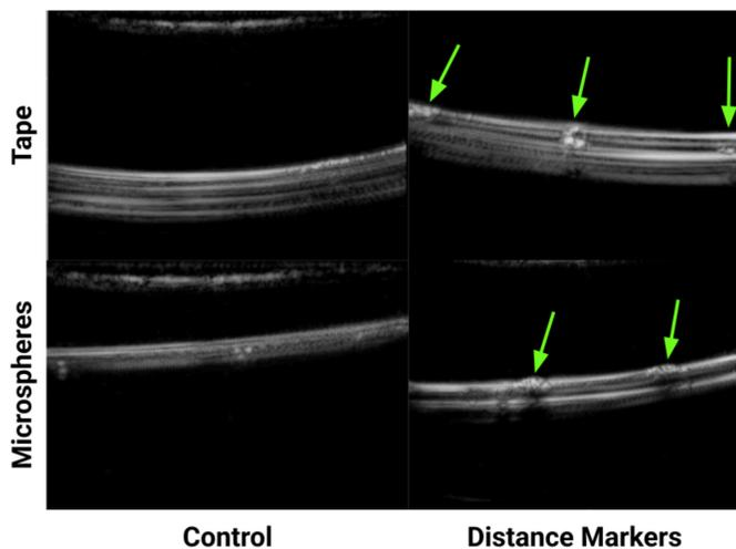
**Figure 4: Ultrasound Images of Experimental Conditions applied to standard UVCs.** Foam material and Microsphere-Urethane coating were applied to a standard UVC. The applied material is seen on the catheter body (as indicated by the arrows).
