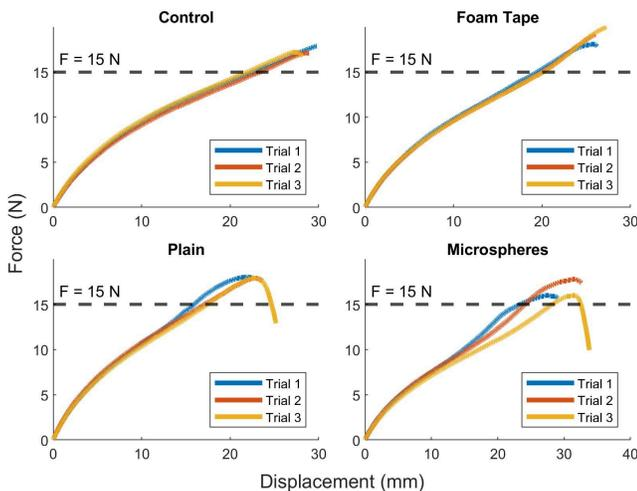
**Figure 2: Tensile Testing Analysis.** Each prototype was stretched with a displacement rate of 20 mm/min and all were able to withstand 15 N of force without failure.
