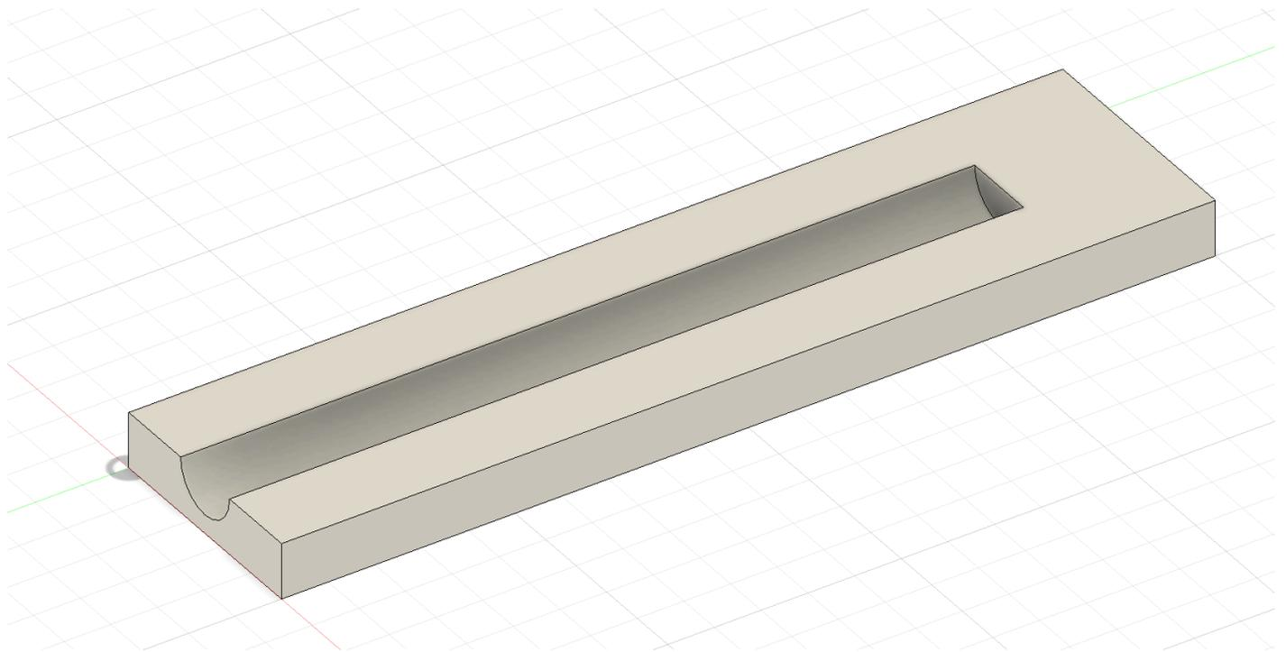
**Supplemental Figure 1: CAD Model of Prototype Mold.** Two copies of this mold were 3D-printed and secured together to hold the tubing while the silicone cured around it.
