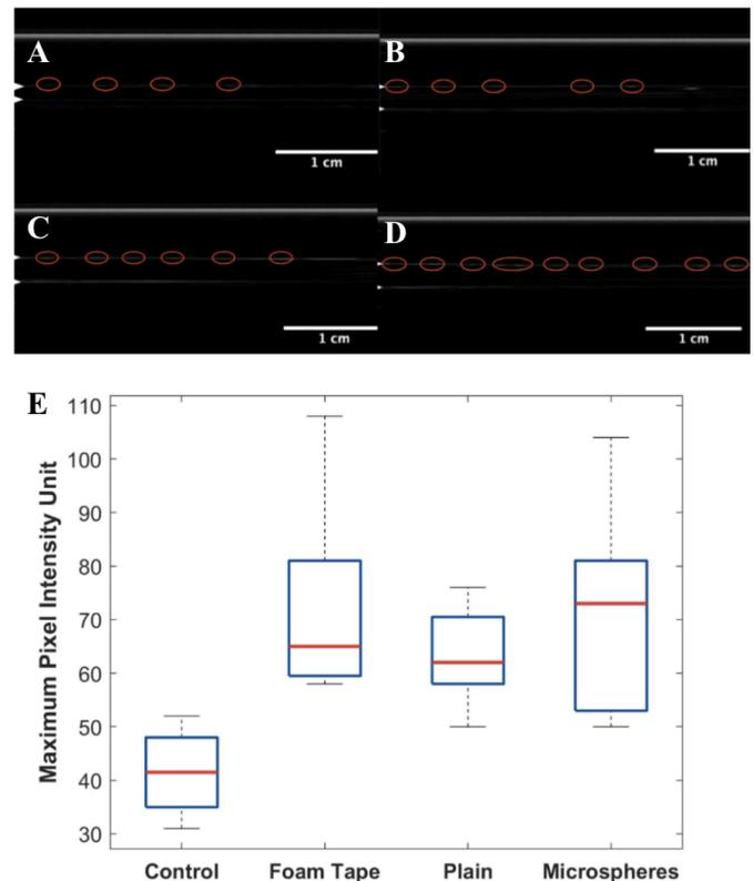
**Figure 1: Analysis of Ultrasound Images.** The Ultrasound Images of Control (A), Foam Tape (B), Plain urethane coating (C), and Microspheres (D) are shown above with red circles indicating the areas with increased PIU units. The maximum PIU of each area was obtained and is expressed in the boxplot (E).
