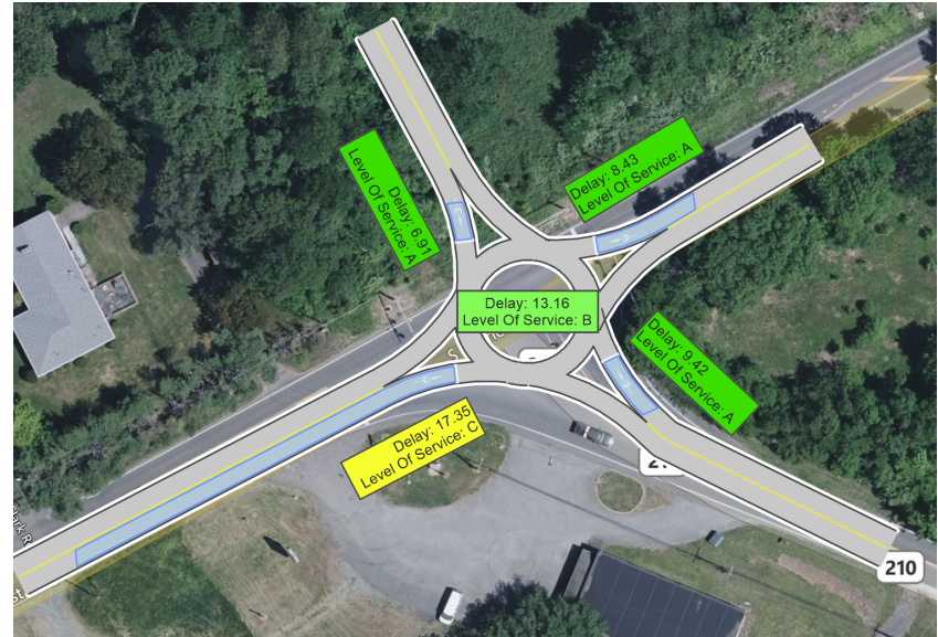
Figure D23: Roundabout PM
