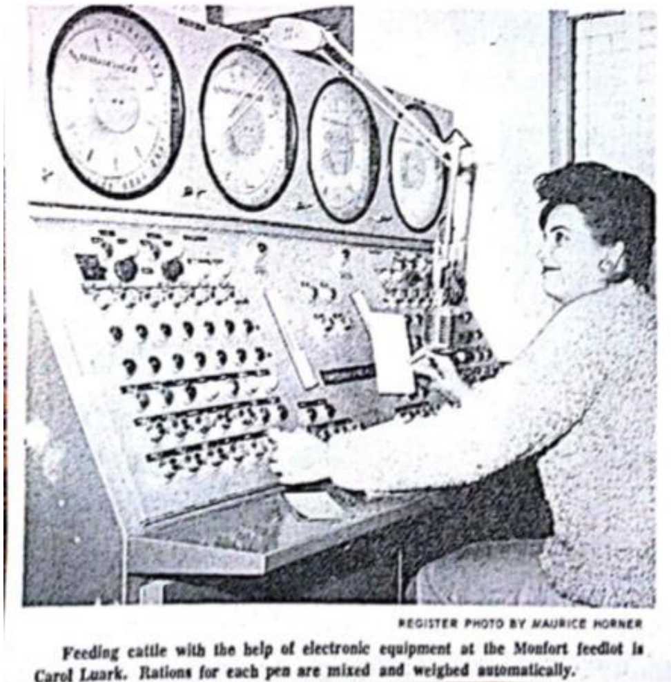
Image 4: Carol Luark, a Monfort employee, inserting an IBM punch card into the computerized equipment at the Greeley feedlot's control room. Source: Ronald Harley, "Giant Feedlot: A Threat to Iowa Farmer" Des Moines Sunday Register (Oct. 17, 1965)
