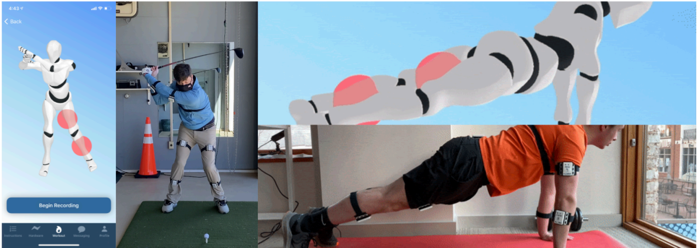
Fig. 1. Images of testing custom motion capture wearable. The wearable was tested on both a member of the Brave Virtual Worlds team and a golfer at The Club at Glenmore to determine spatial and motion data functionality relative to the real world. The images depict both a person wearing the wearable along with a 3D representation on a custom mobile application developed for the device.
