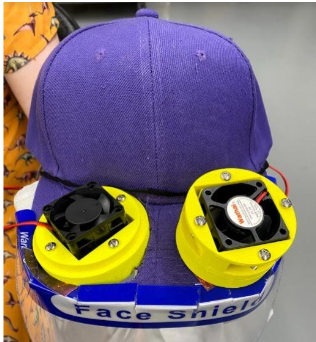
Figure 7: The second prototype with the two kinds of fan casings attached.
