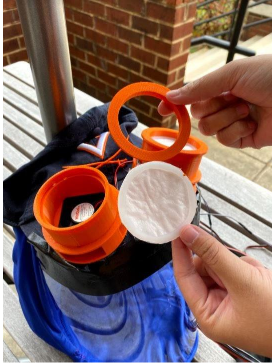
Figure 12: Removable Filter Material and Top Section of Fan Casing
