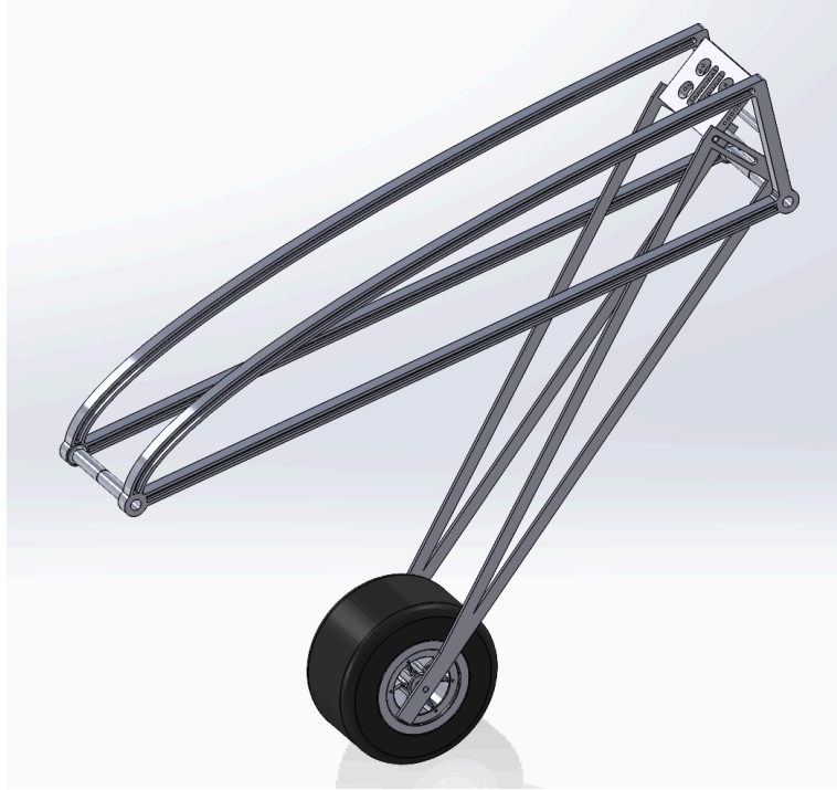
Figure 15: Landing gear Design
