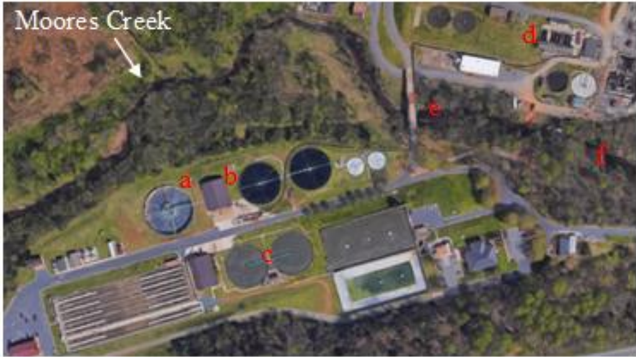
Figure 2: Map of Sampling Locations at the Moores Creek Wastewater Treatment Plant: Possible sampling locations include multiple areas within the wastewater treatment process (a-d) as well as along Moores Creek on both sides of the final effluent outflow (e-f) (Google map adapted by Sutton, 2019).
