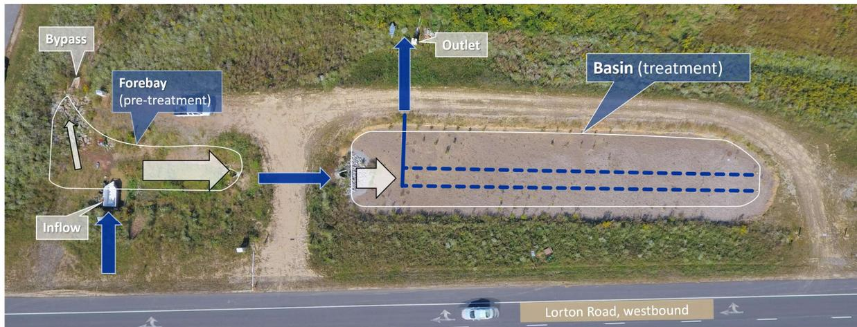
Figure 2.2. Aerial image of bioretention with piped flow represented by dark arrows, surface flow represented by light grey arrows, and perforated underdrain represented by dotted lines.
