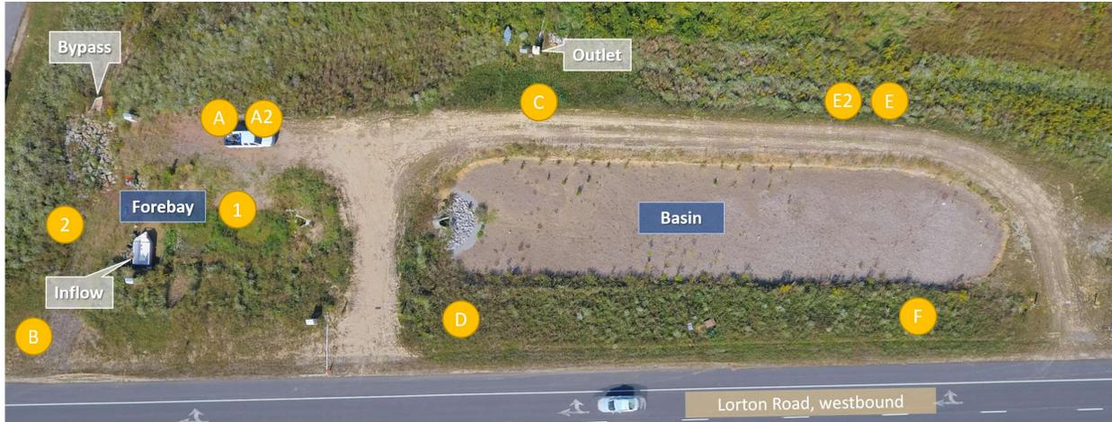
Figure 3.1. Location of wells around bioretention. Well 1 and Well 2 were drilled manually by auger and all others drilled mechanically.
