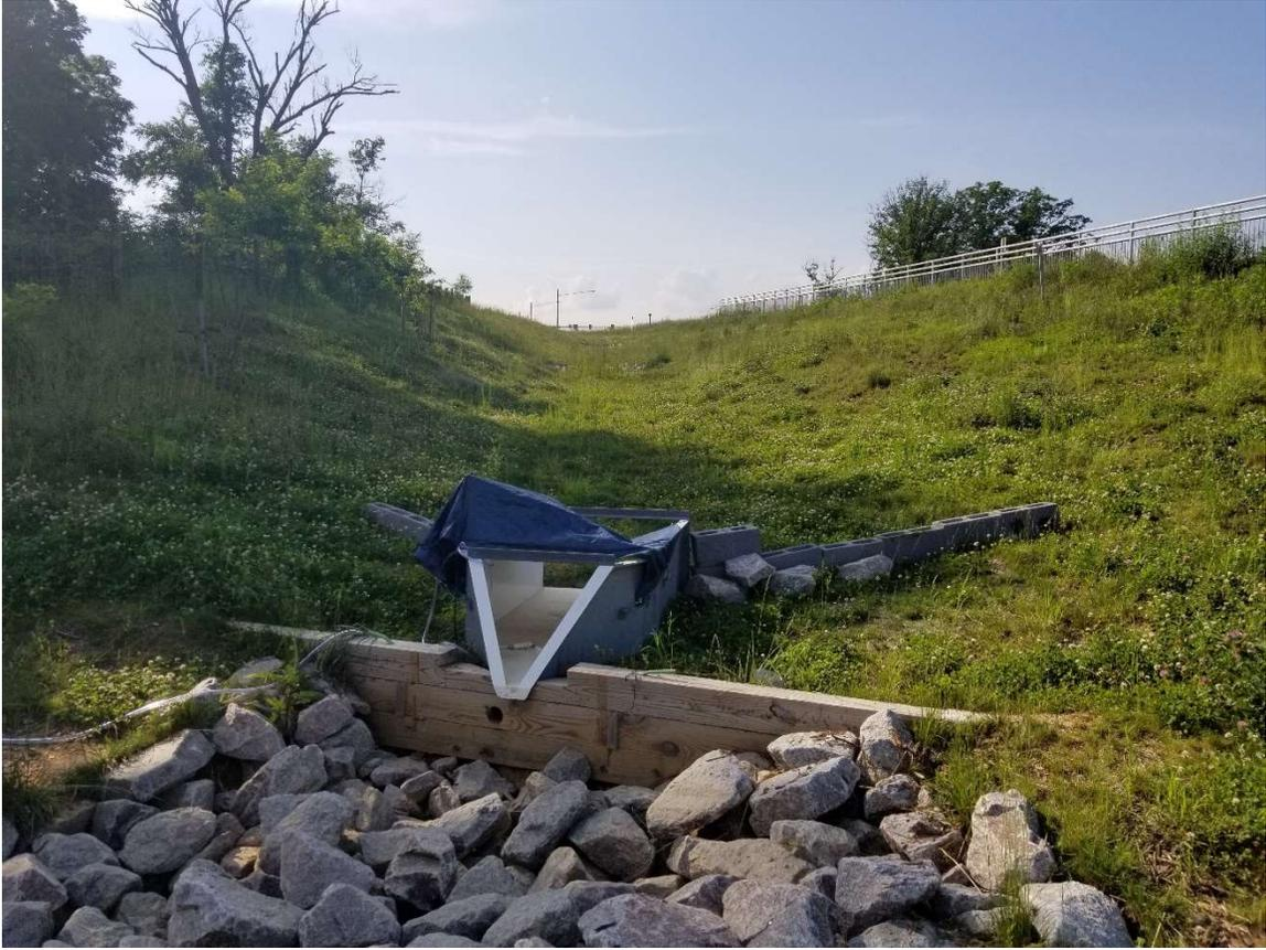
Figure E.1. Grass channel flume with cinder blocks preventing flow-around
