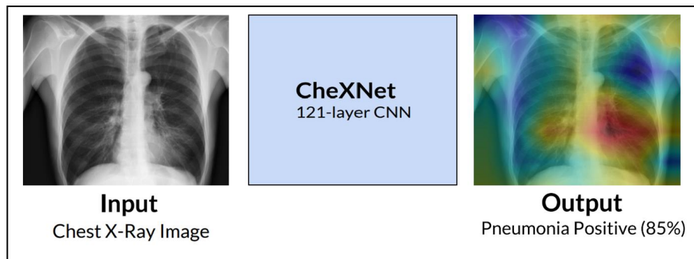
Figure 2: CheXNet takes in the chest x-ray as the input and outputs the location of where pneumonia is the most severe, show in red at the lower left lobe (Rajpurkar et al., 2017).
