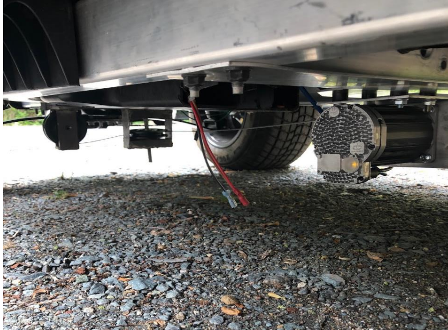
Figure 10: Installed Clearpath MC Brake Motor. (Patrick Dunnington, 2023)
