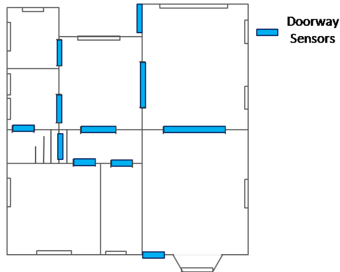
Figure 4.3: Eleven doorways were instrumented for data collection. Of them, two were external doors and two led to other floors.
