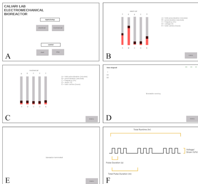
Figure 5: Graphical User Interface (GUI) Panels (A) Menu page for navigating display (B) Electrical value input page (C) Mechanical value input page (D) Bioreactor start and monitoring page (E) Bioreactor stop page (F) Graphical representation of electrical and mechanical stimulation input values
