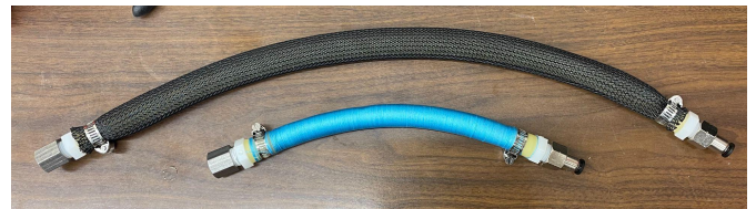
Fig. 14. Final McKibben Muscle Design (top) and Fishing Line Model (bottom)
