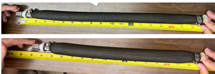
Fig. 16. McKibben Muscle Change in Length Test
