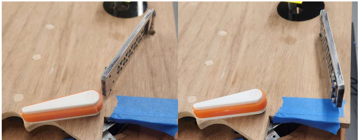
Fig. 2.5.2. Diverter gate in closed and open position
