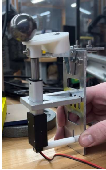
Fig. 2.6.5. Testing of the final trapdoor assembly
