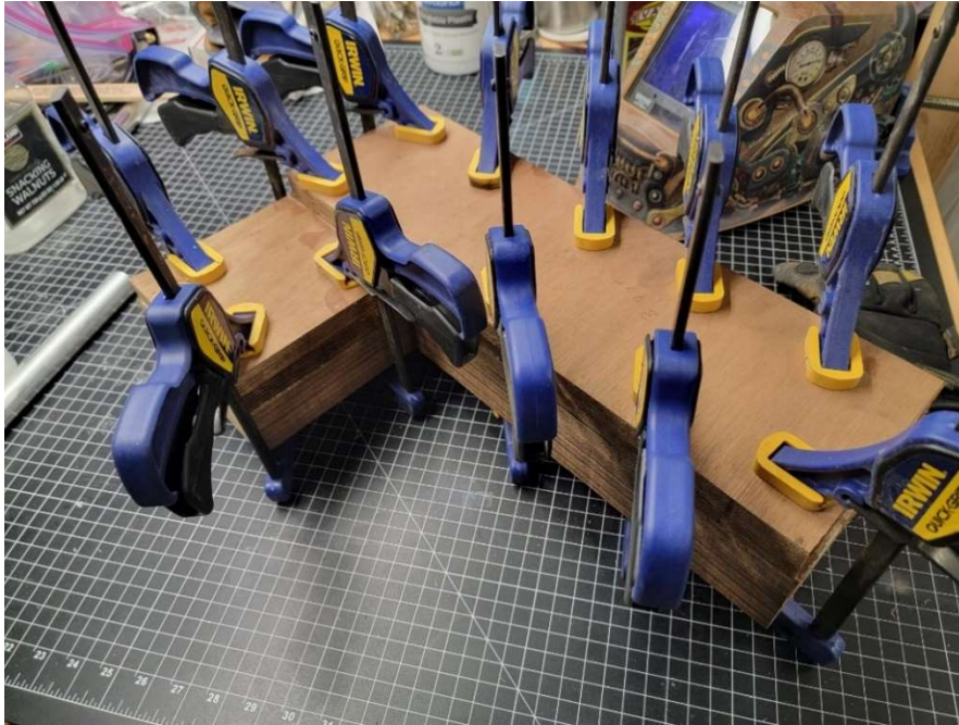
Fig. 3.3.4. Upper Playfield Plywood Stock Glued
