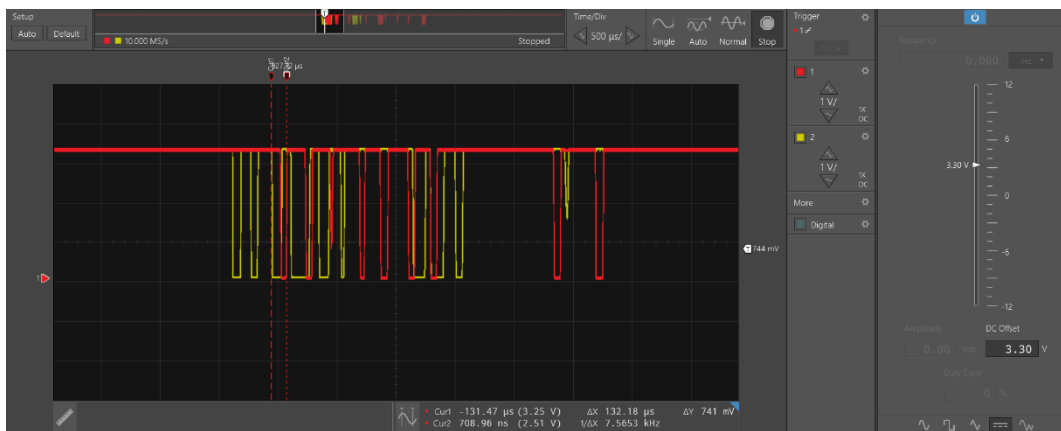
Figure 3941 - Verification of Both Piezos Output
