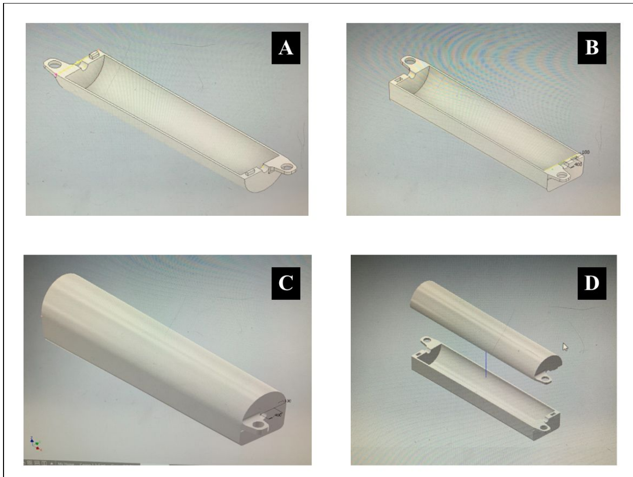
Figure 6: Screenshots of the final linear generator casing design developed on Autodesk Inventor 2019.
