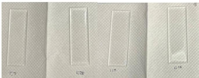
**Figure 6. Crosslinking experiment.** Elastomer to curing agent ratios tested were 5:1, 10:1, 15:1, 20:1.
