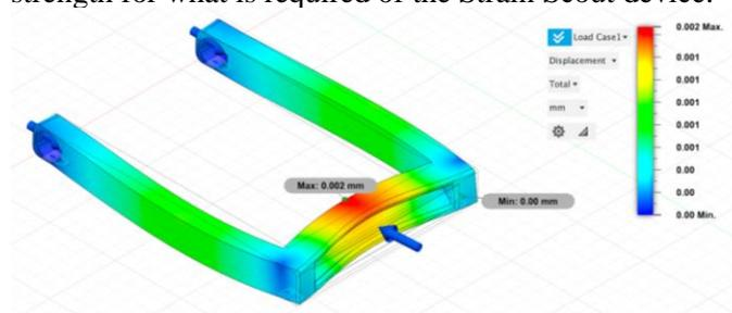
**Figure 4. Strain Testing.** Finite element analysis (displacement with strain of membrane) with aluminum scaffolding.
