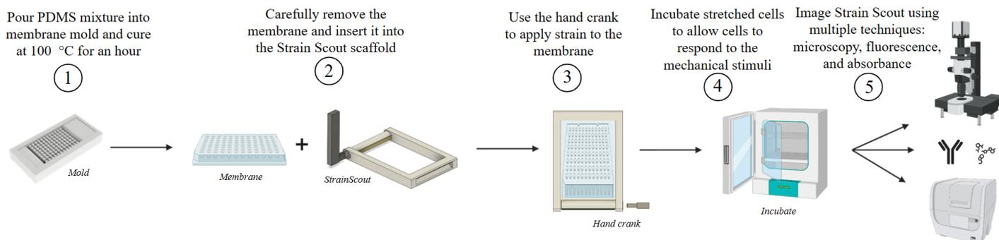
**Figure 1. Intended procedure for Strain Scout.** Utilize a mold to produce a PDMS membrane and insert the membrane into the Strain Scout Scaffold. Seed cells of choice and incubate before and after applying strain. Image with antibodies or small molecules to identify relevant mechanotransduction pathways.
