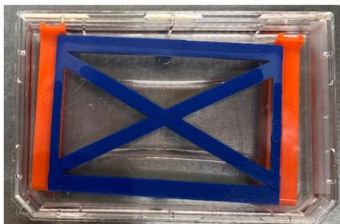
**Figure 2. Previous Strain Scout Design.** The membrane in this image is stretched. At the halfway point, posts protrude and act as an anchor for the membrane clips (orange) when the previous version of Strain Scout is in an unstretched state.
