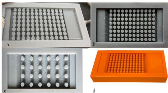
**Figure 5. Iteration of the Strain Scout membrane mold.** a) Original large 96-well plate design with PDMS and made out of resin b) Scaled down design (0.7 scale) c) 24-well plate membrane mold d) Scaled down (0.7 scale) mold made out of ABS and with increased tab length.
