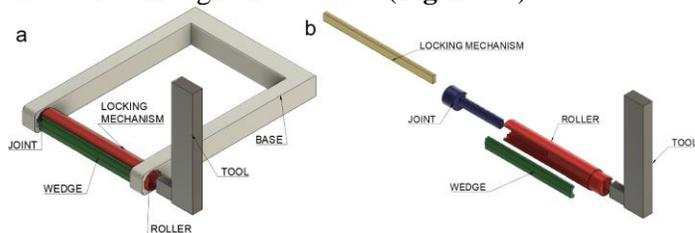
**Figure 3. Final Strain Scout Scaffold Design.** a) Final labeled drawing of Strain Scout device using Fusion 360 b) Exploded drawing of stretching mechanism using Fusion 360
