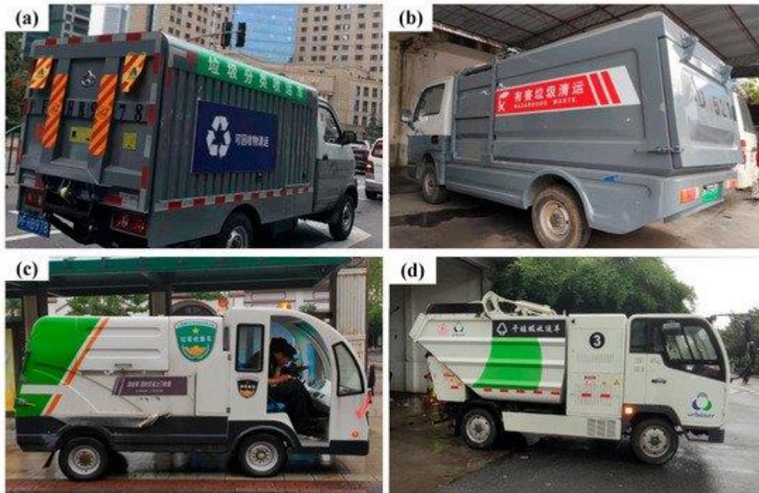
Figure 2. Transportation vehicles of different categories of waste: (a) recyclable waste, (b) hazardous waste, (c) wet waste, (d) dry waste.
