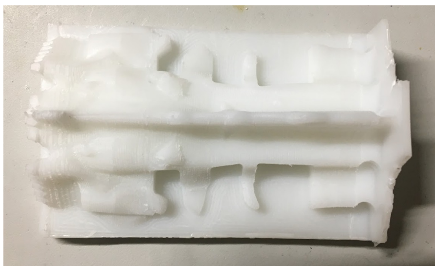
Supplemental Figure 4: The figure shows the continuation of the commercialization phase. The silicone mold will be replaced by a 3D printed part. Eventually, the 3D printing process will be contracted to an outside vendor to increase reliability and speed of production.
