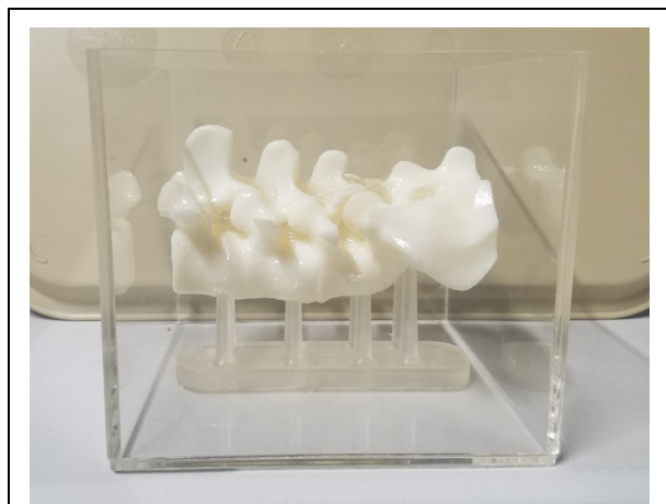
Figure 5: This figure shows a 3-D printed spine with a backfilled spinal canal adhered to a stand inside the prototype box. This demonstrates what the box looked like prior to pouring the skin and tissue layers.
