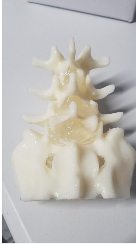
Supplemental Figure 6: The image depicts the backfilled spinal canal. The spinal canal was backfilled with polyurethane. This was done to make the phantom spine more similar to the in vivo human spine.
