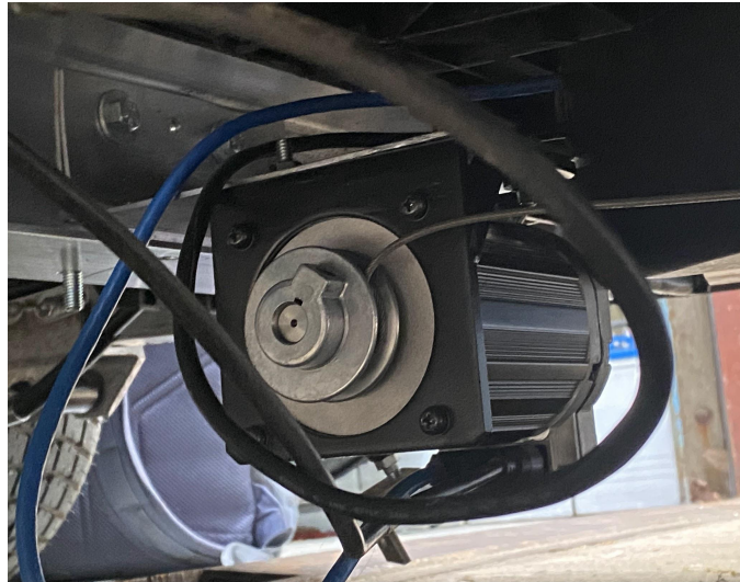
Figure 17: ClearPath Servo motor used for braking system on Cart 789 with motor mount attaching it to the steel bracket underneath the cart.
