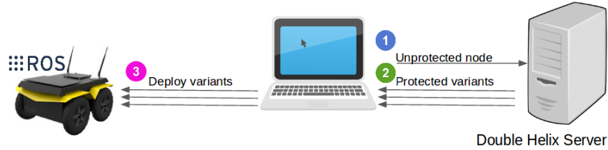
Figure 3.3: Generating and deploying Double Helix variants into our ROS based UGV
