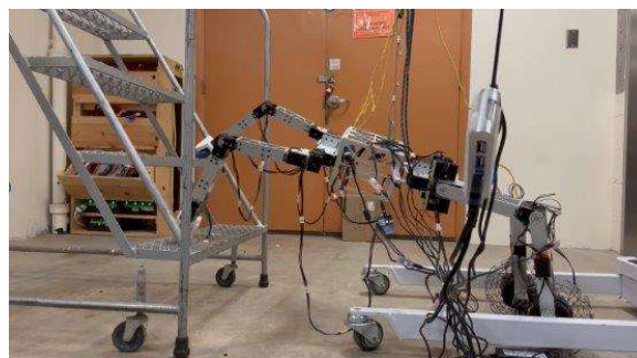
Figure 16: Upper Body Climbing Test
