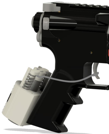
Figure 30. Trigger mechanism attached to Airsoft handle.
