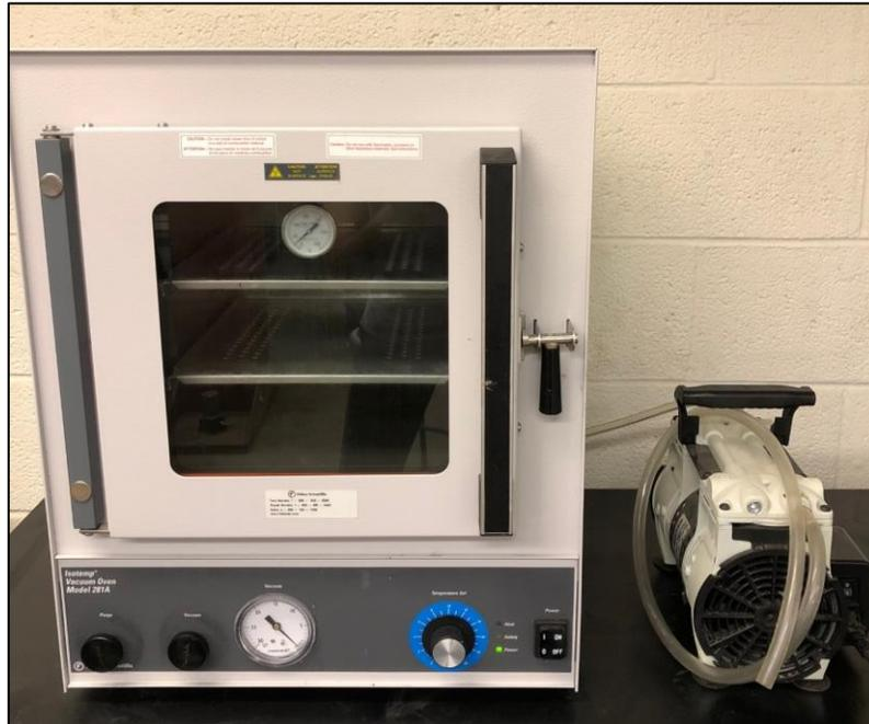
**Figure 7:** Vacuum oven and vacuum pump
